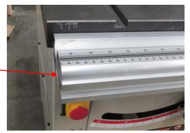
Find the Rip fence assembly complete with the Side extension plate. Remove the fence extension side plate off the fence and put it aside.
