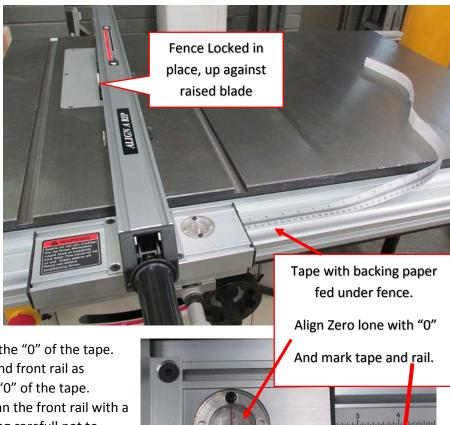
Start peeling the backing tape off the new tape and position the tape on the rail, lining up the black marker lines as you go, then if all Ok, peel the rest of the backing paper off as you put the rest of the tape into the groove. Press the tape down firmly along its lengh.
