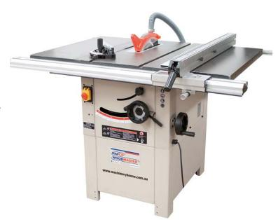
**SET UP #2** With both extension tables on the Right hand side and the support leg supplied used to prop it up.
