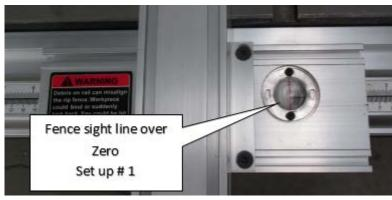
For set up # 2 Remove the existing measurement tapes 0-64 on the left and 0-62 on the right of the front fence rail as these are only needed for set up #1. The tape can be carefully lifted with a sharp blade and peeled off. Residue glue on rail can be removed with kerosene and a small scraper.
