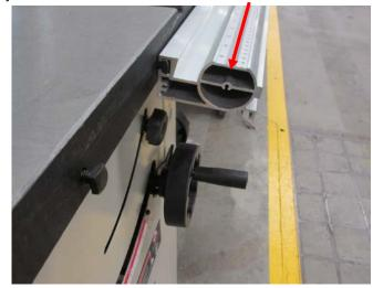
For set up #2 Align each rail so it is in from the left edge of the main cast table about 8 to 10mm
